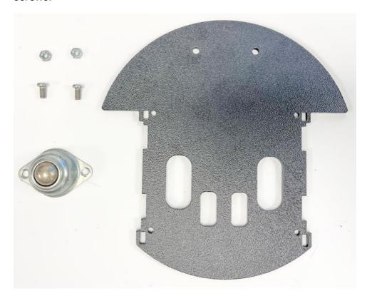
Install metal-ball wheel on the bottom chassis plate.
