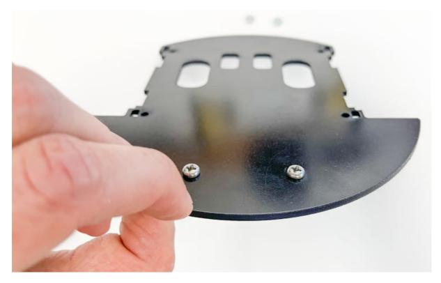
Then use M3 nuts to fix screws.
