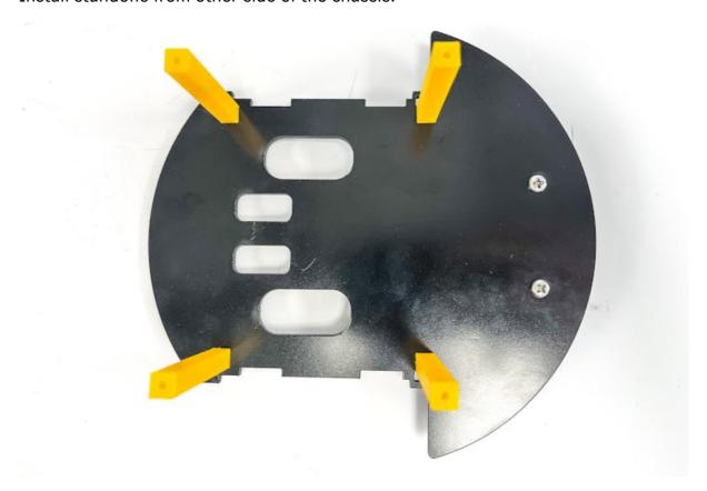
Make sure that standoffs are aligned with the slots on the chassis.
