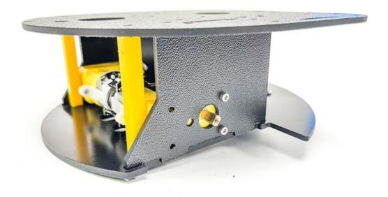
Now fix it using four M2.5x10 mm screws.
