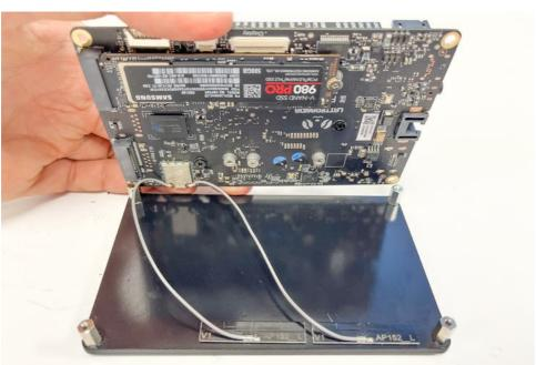
Finally mount board using x4 M2.5x6mm screws.
