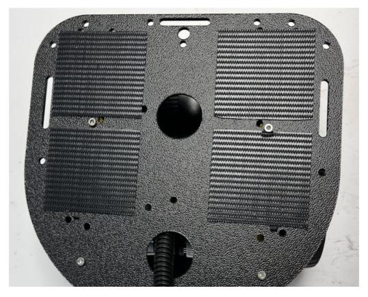
Take Velcro soft side the loop and put it on the bottom side of the power bank.
