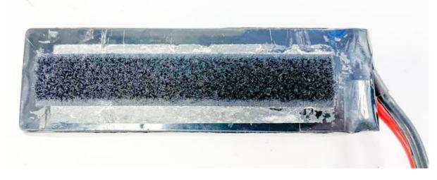
Turn it over and stick Velcro tape with hooks on the top side.
