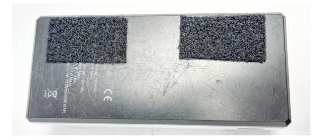
Now stick a Velcro tape with loops on the 2S-battery bottom side.
