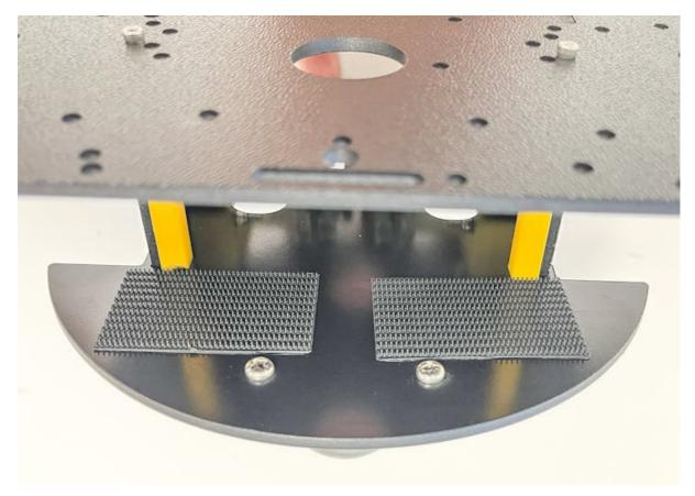
Now stick Velcro tape hooks on the top chassis plate.
