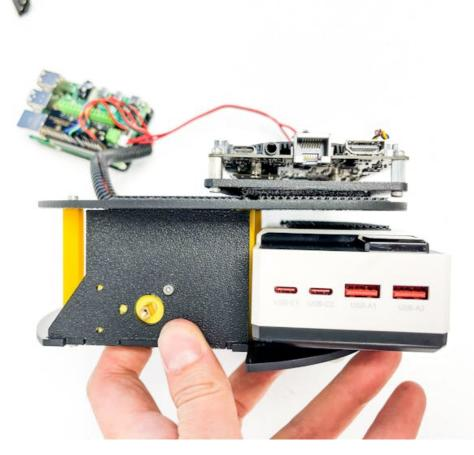
After that install Li-Po batter on top.
