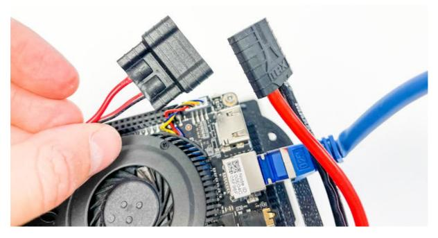
It will power-up motor driver and Raspberry. Motor driver has accept voltage in range 7-12V.
